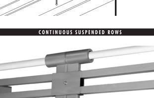
For two or more pendant fixtures mounted end to end, order and install **SDC** swing double connector to align fixtures and prevent interfixture collision.
